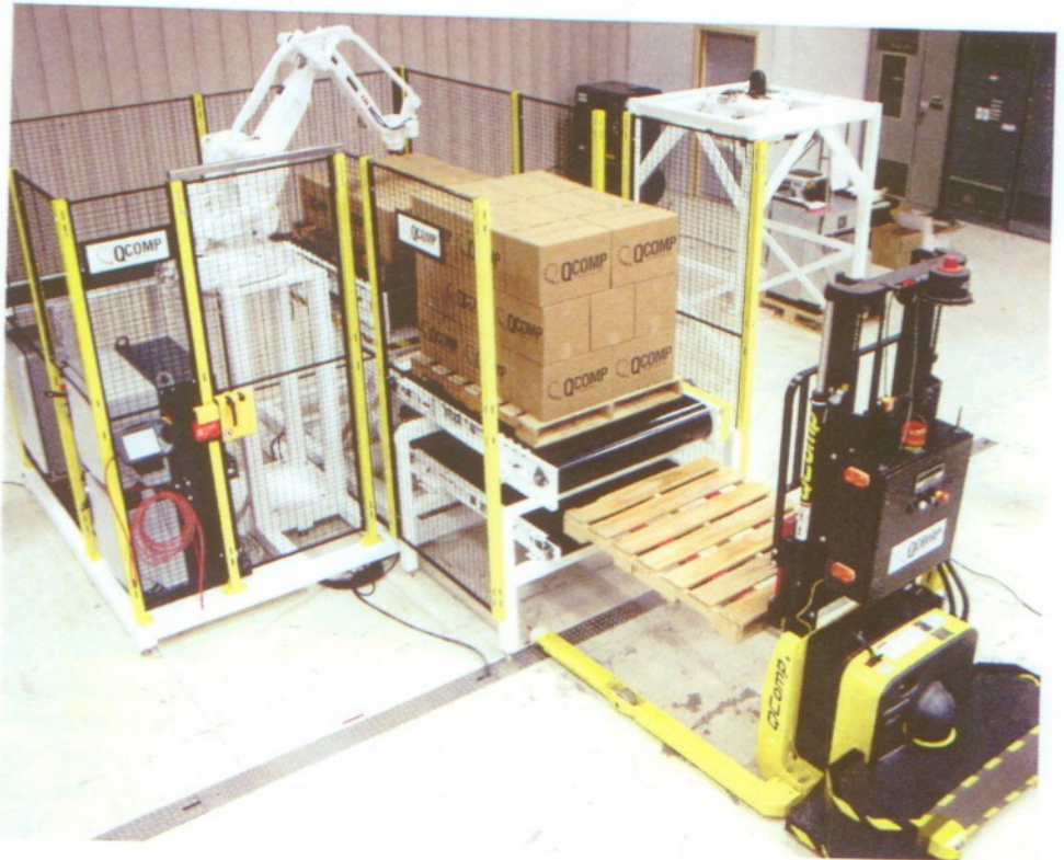
Photo courtesy of QComp Technologies THIS AUTOMATED PALLET STACKING ROBOT CAN EASILY MOVE MATERIAL AROUND A WAREHOUSE.
